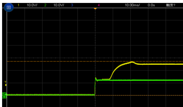
Figure 6, Output voltage established ( I_{out} = 1\text{A} )
