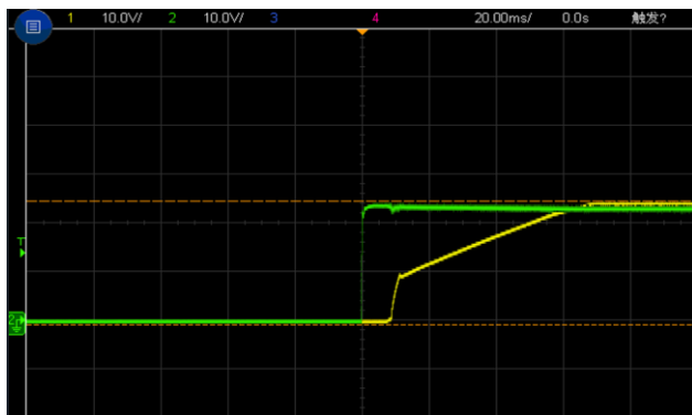
Figure 6, Output voltage established ( I_{out} = 30\text{A} )
