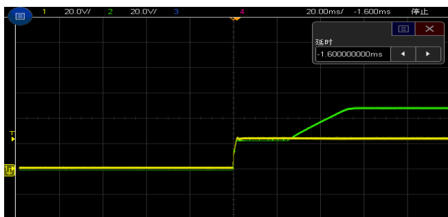
Figure 6, Output voltage established (Iout = 10A)
