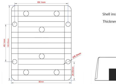
Shell installation diagram Thickness : 39mm
