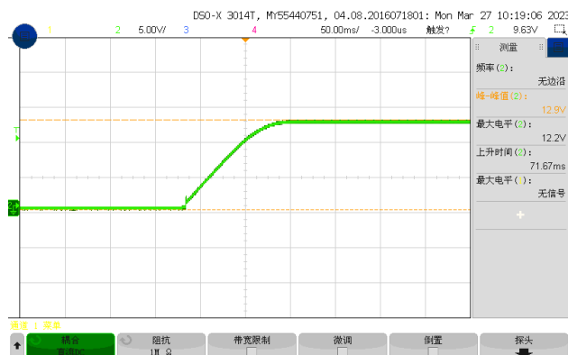
Figure 6, Output voltage established (Iout = 10A)
