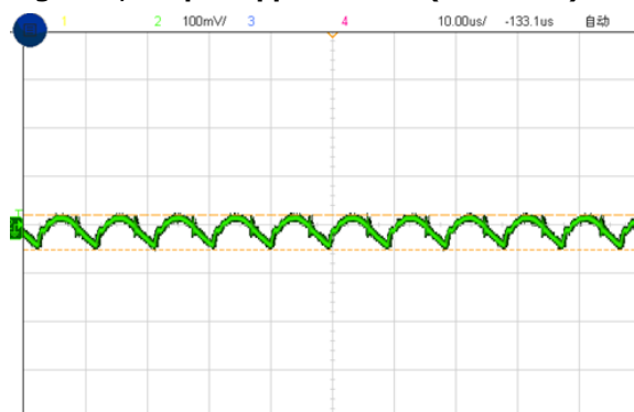
Figure 7, Output ripple & noise ( I_{out} = 3\text{A} )
