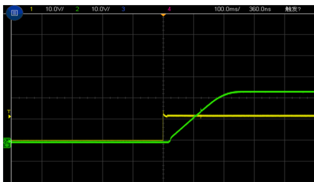
Figure 6, Output voltage established ( I_{out} = 10\text{A} )
