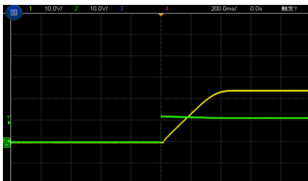
Figure 6, Output voltage established ( I_{out} = 15\text{A} )
