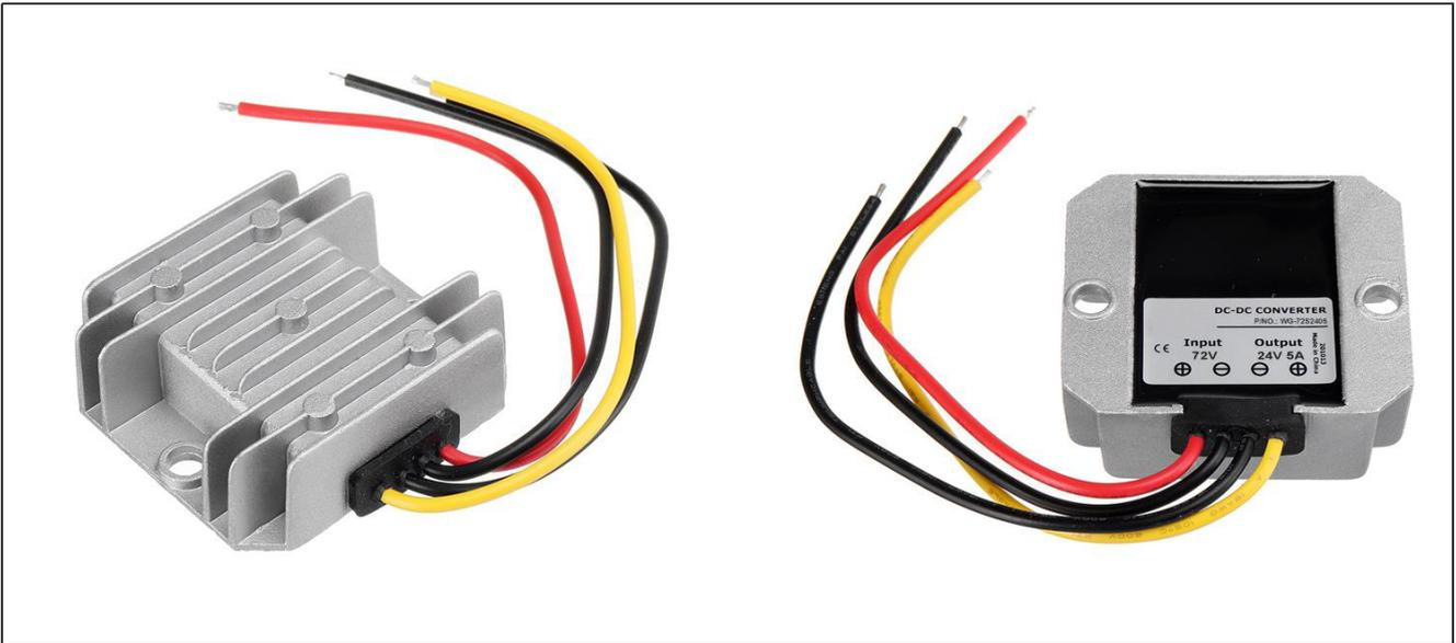
The WG-72S2405 is a Non-isolated DC-DC converter that uses a synchronous rectification technology, and features high efficiency and power density. It has the dimensions of 64mm x 57mm x 22mm (2.52 in. x 2.24 in. x 0.87 in) and provides the rated output voltage of 24V and the maximum output current of 5A.
