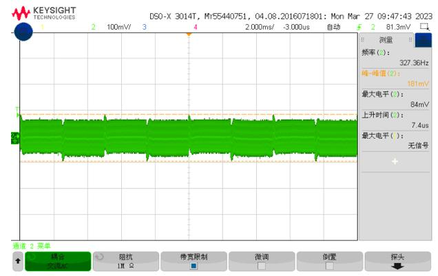
Figure 6, Output voltage established (Iout = 5A)
